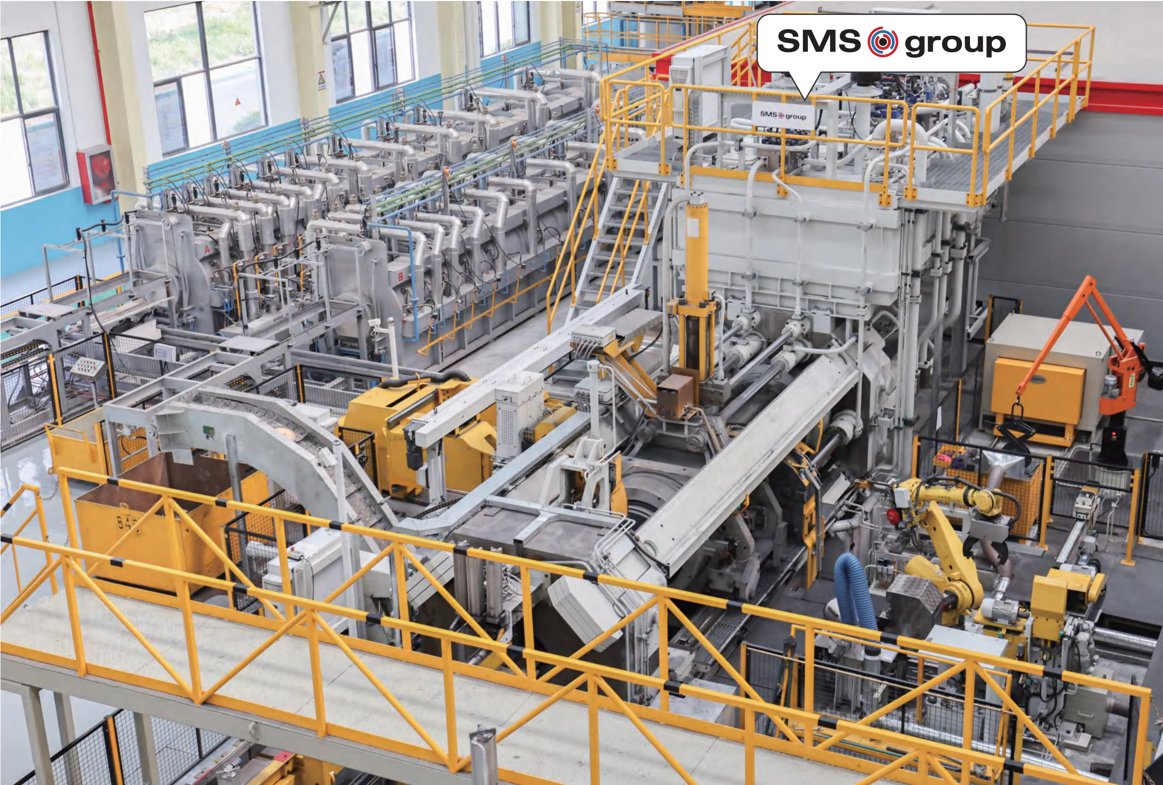
西马克铜及铜合金2800吨反向挤压生产线 28MN Indirect Extrusion Press Line for Copper and Copper Alloys
