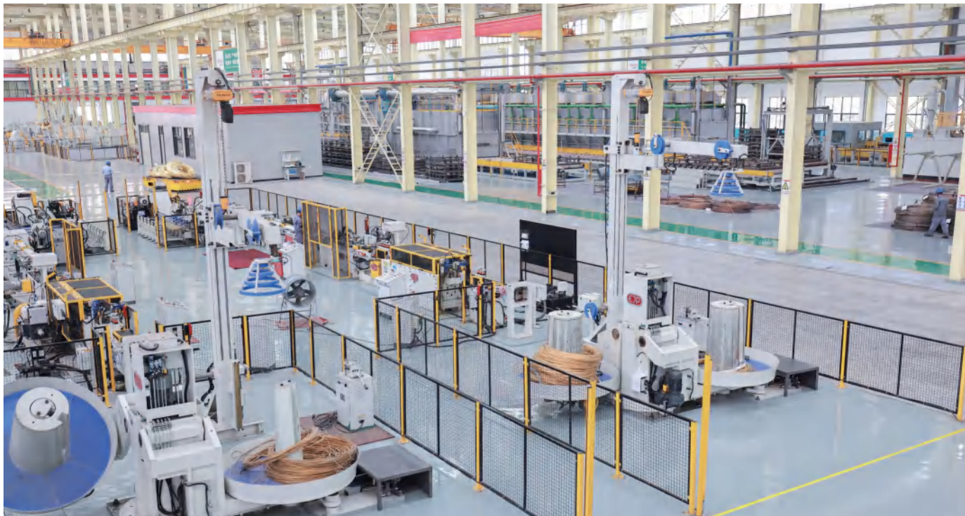
铜及铜合金2.5吨EJP联合拉拔机生产线 2.5T EJP Drawing Machine Line for Copper and Copper Alloys
