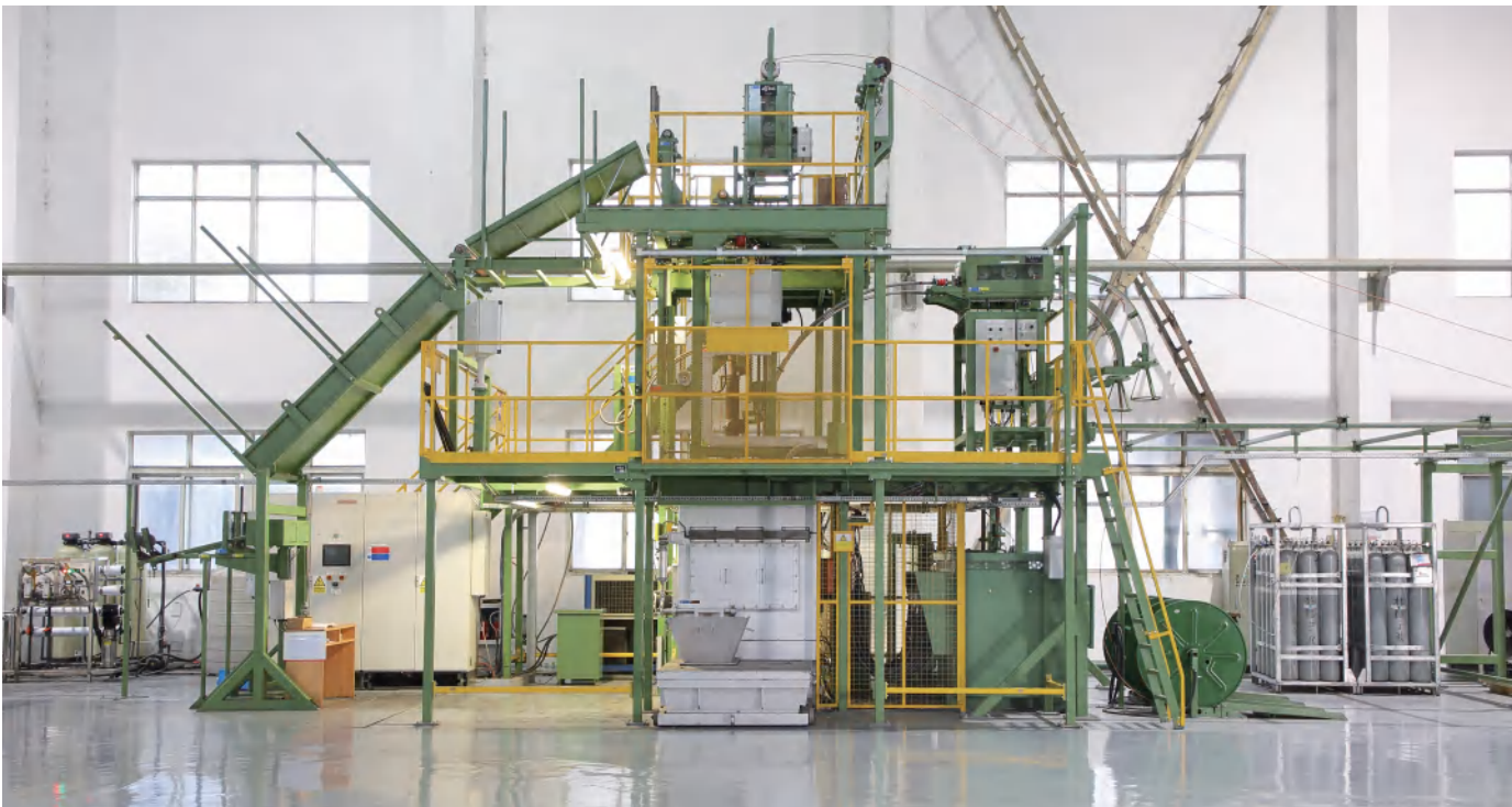
劳同美德上引连续铸造机 Rautomead Upwards Vertical Continuous Casting Machine
