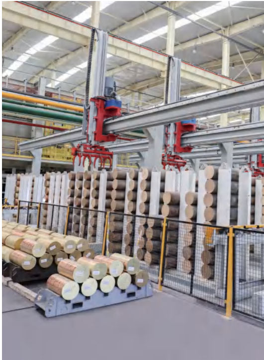
铜锭智能库 Intelligent billet warehouse
