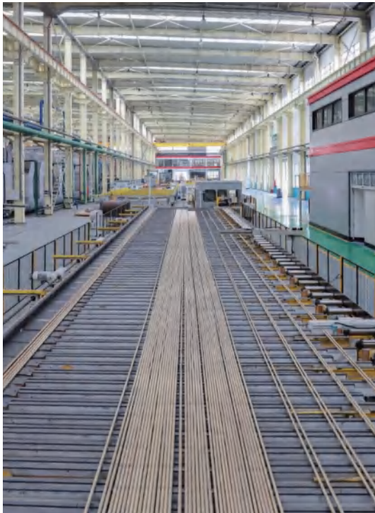
30米冷床 30m cooling bed
